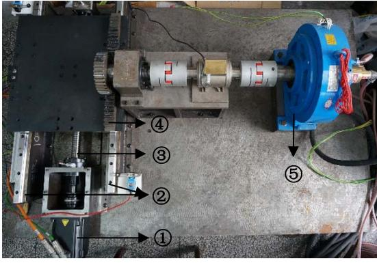
Figure 4. Degradation test bench for ball screw
