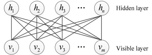
Figure 1. The structure of RBM
